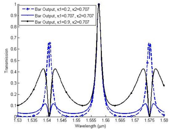
Fig. 6. Transmission at port 2 through the device at different coupling coefficients  $\kappa_1$ ,  $R_1 = 5\mu\text{m}$ ,  $R_2 = 10\mu\text{m}$
