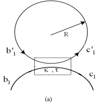
Fig. 2 Schematic diagram of a microring resonator
