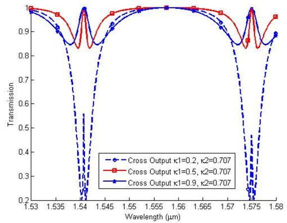
Fig. 5. Transmission at port 2 through the device at different coupling coefficients  $\kappa_1$ ,  $R_1 = R_2 = 5\mu\text{m}$
