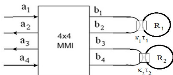
Fig. 1 Schematic diagram of a 4x4 MMI coupler based device
