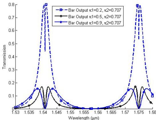
Fig. 4. Transmission at port 2 through the device at different coupling coefficients  $\kappa_1$ ,  $R_1 = R_2 = 5\mu\text{m}$
