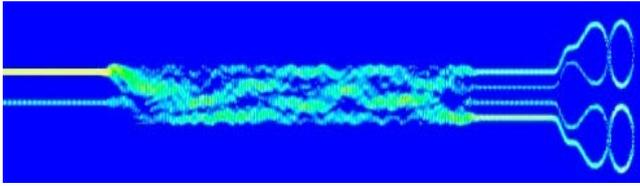
Fig. 3 FDTD simulations for 4x4 MMI coupler for input 1, output port is at port 2
