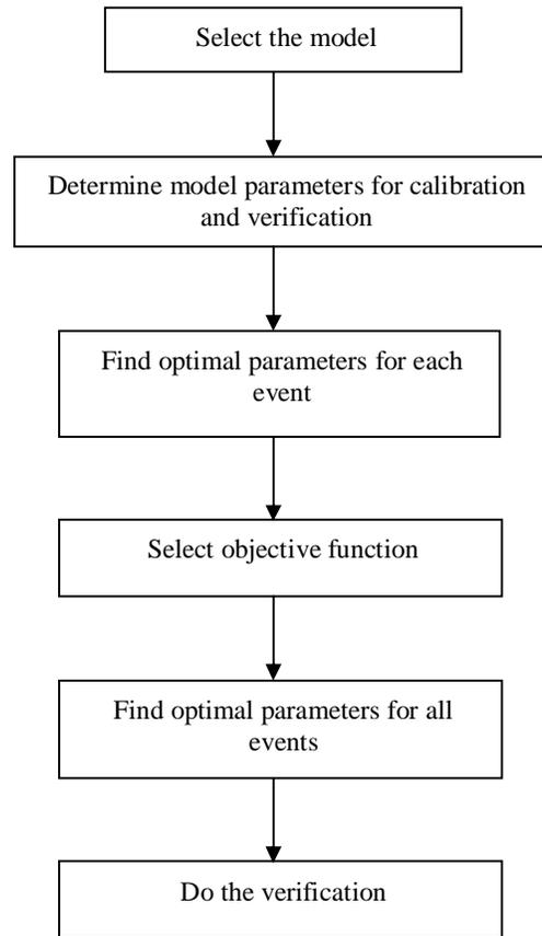
Figure 2.1. Procedure for parameter calibration and verification.
