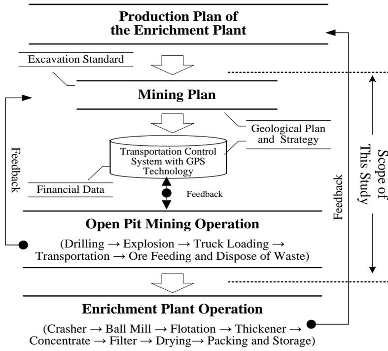
Figure 1: Simplified process map for open pit mining operation in Company "A"
