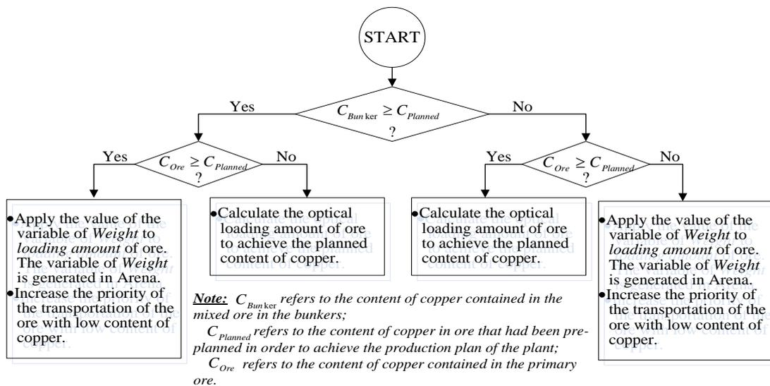
Figure 4: Algorithm for calculating load capacity when dispatching trucks to excavators
