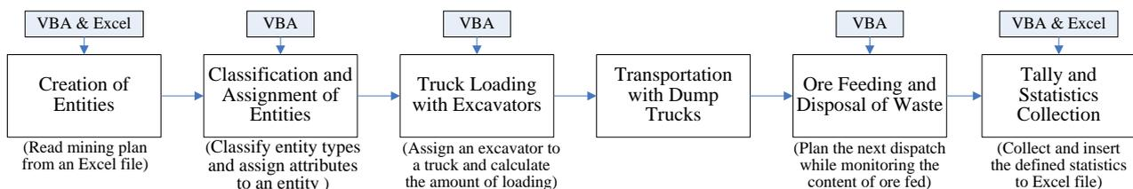
Figure 2: Overall structure and simulation model flow
