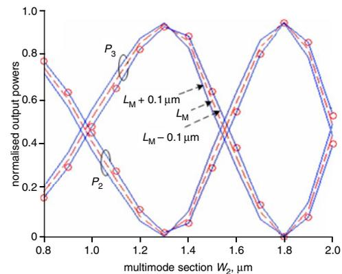
Fig. 3 Normalised output powers against multimode section width for different MMI linking section lengths
